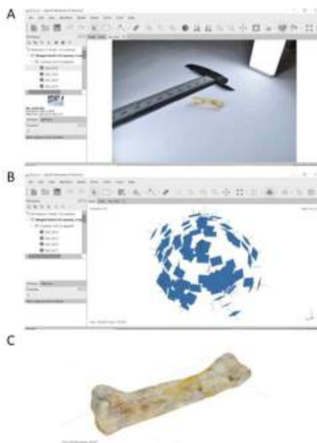
Figure 2: Generating a 3D model of the Otavipithecus namibiensis second manual phalanx using photogrammetry. After loading photographs into the software [A], the positions of the photographs are estimated [B] and the object is reconstructed in 3D [C].
